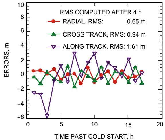
Fig. 7. The real-time orbit using onboard data from GPS/Met on July 16, 1996 (Case 1).
