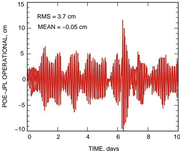
**Fig. 1. The JPL TOPEX/Poseidon daily operational orbits compared with the definitive precise orbits. The operational orbits are available 11 to 17 hours after the last data point.**
