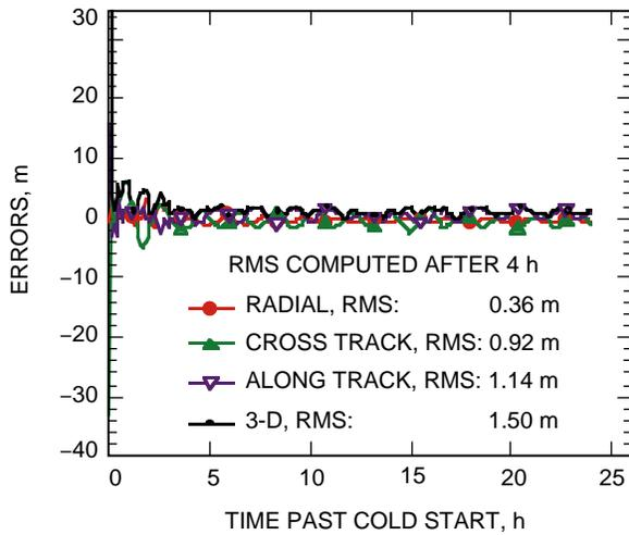
Fig. 6. TOPEX/Poseidon real-time position accuracy with broadcast level GPS orbit errors and enhanced real-time clock errors (Case 1).
