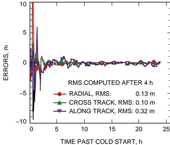
**Fig. 8. TOPEX/Poseidon real-time positioning with precise orbits and clocks (Case 2).**
