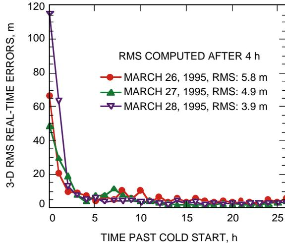
**Fig. 4. The 3-D error after a cold start using broadcast GPS orbits and clocks for TOPEX/Poseidon at a 1300-km altitude.**
