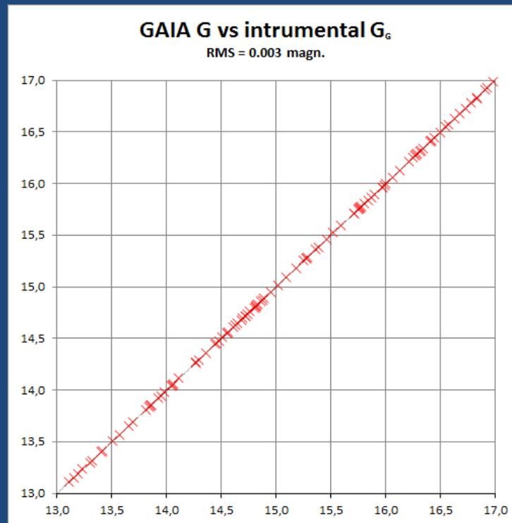
A star of 17 magn. is measured with a 15 s exposure at the 300 mm f/3.3
