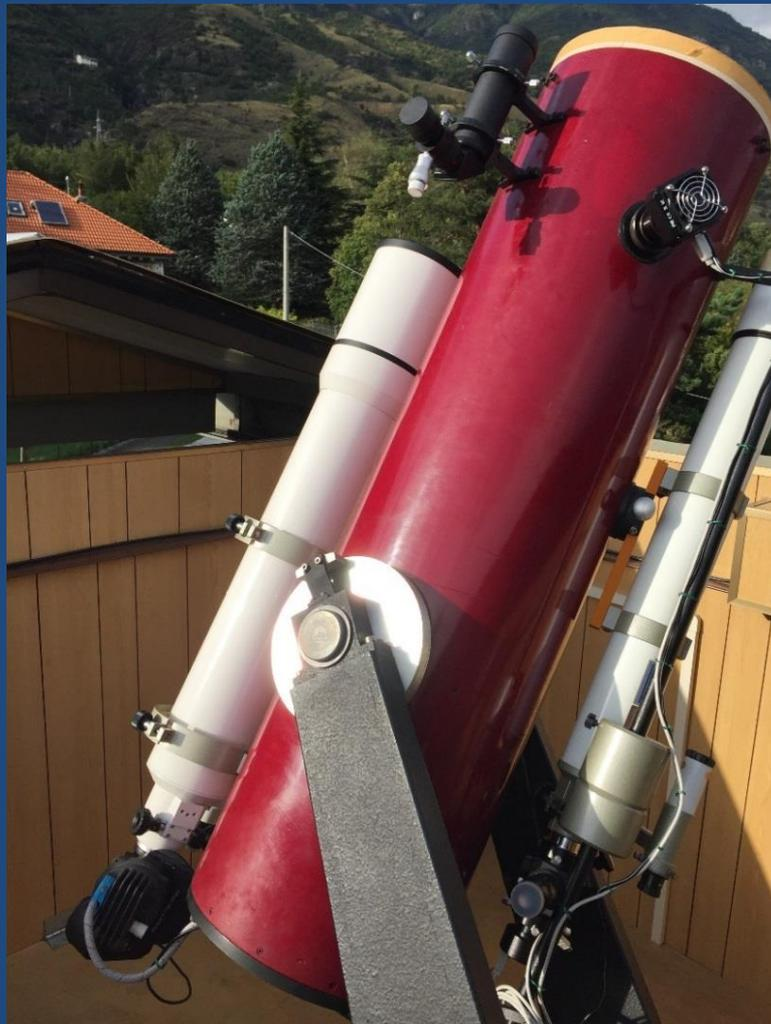
The current layout of the Grange Obs. instrumentation: the main 300 mm Newton reflector is working at  $f/3.3$  with Sloan and GAIA filters, and the piggyback 140 mm astrograph mounts a Johnson BVR photometer.
