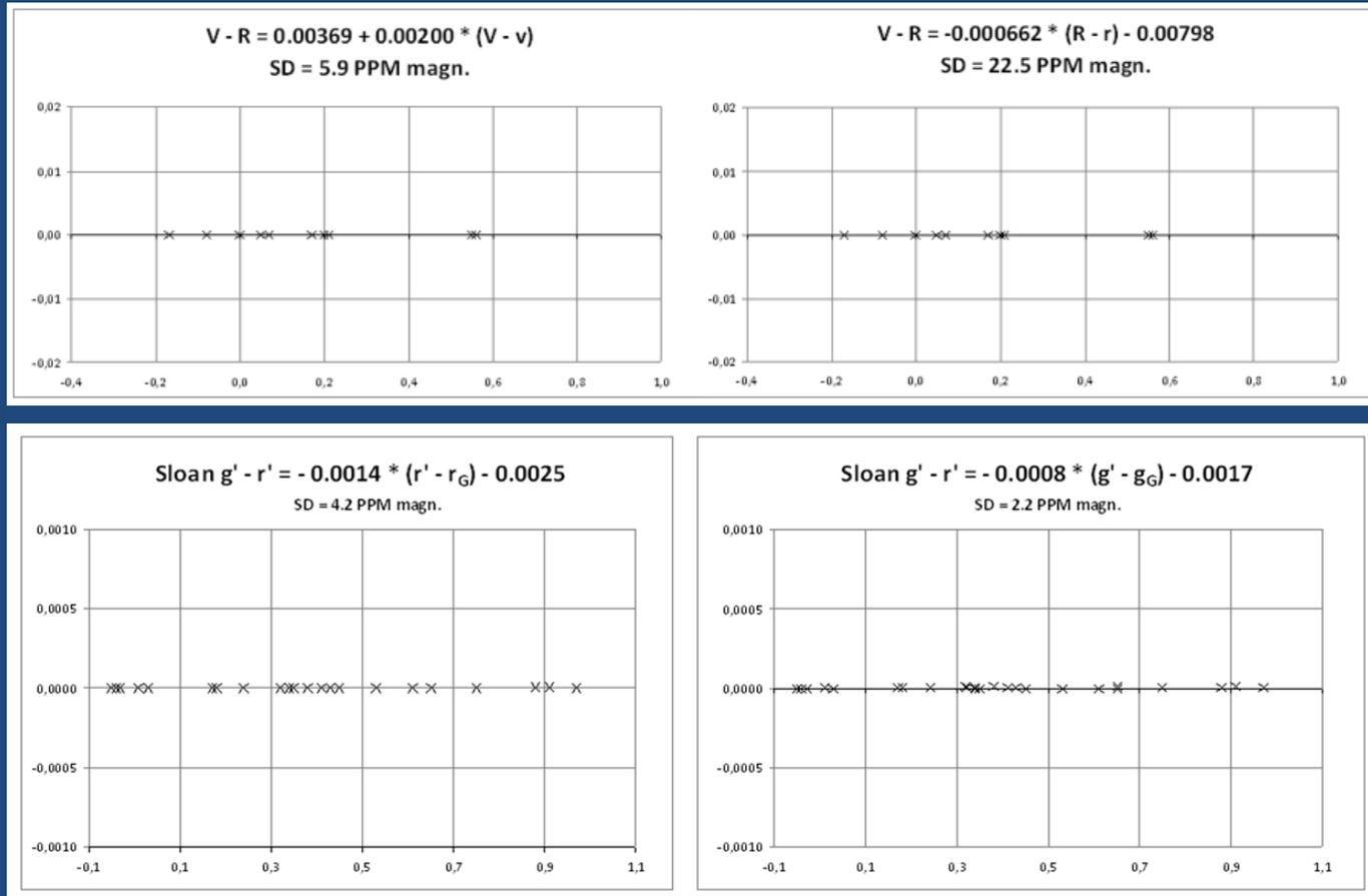
The calibration graphs of the photometric filters developed at the Grange Obs. Color indices can measure stars surface temperature and metallicity index. The photometers can also measure exoplanet transits on stars
